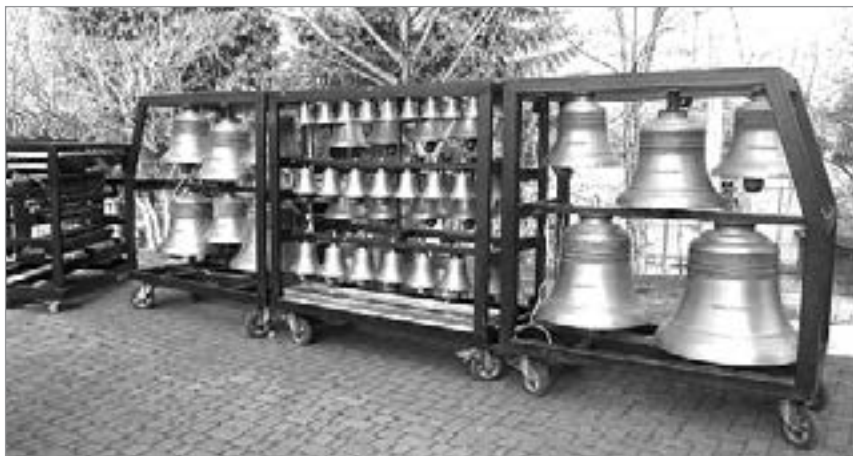
Photo 1. Mobile carillon by Sergei and Leonid Botvinko (50 bells, 2700 kg – Bell-foundry Petit & Fritsen, 2007)
